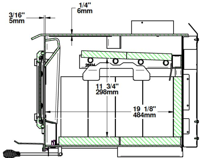
Figure 6: Side View - Combustion Chamber
