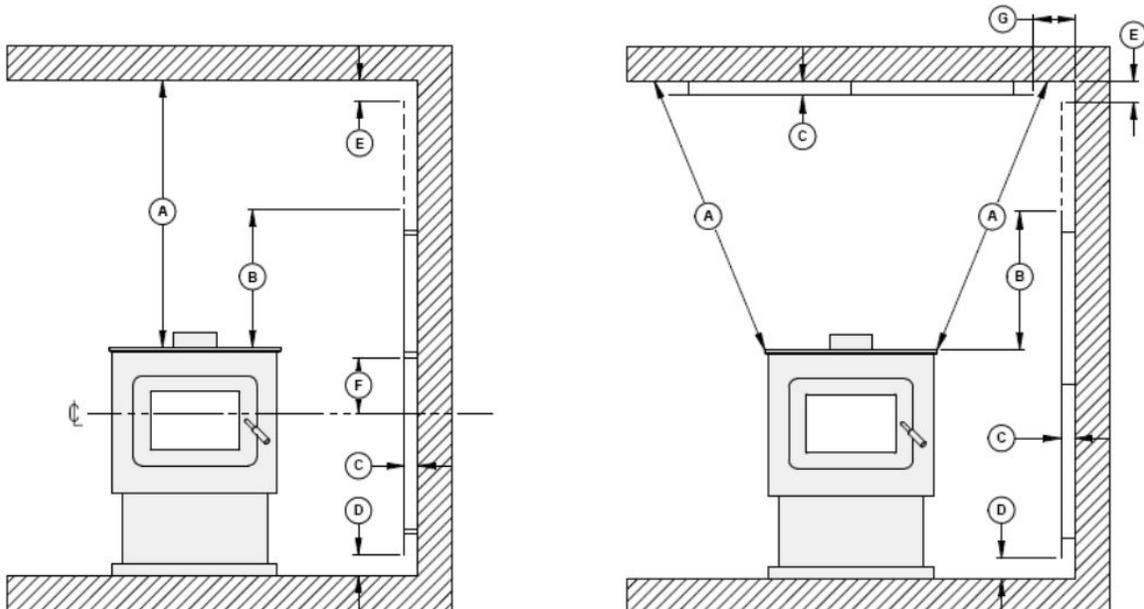
Figure 11: Heat shield clearances
