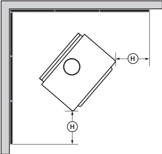
Figure 14: Heat shield clearances
